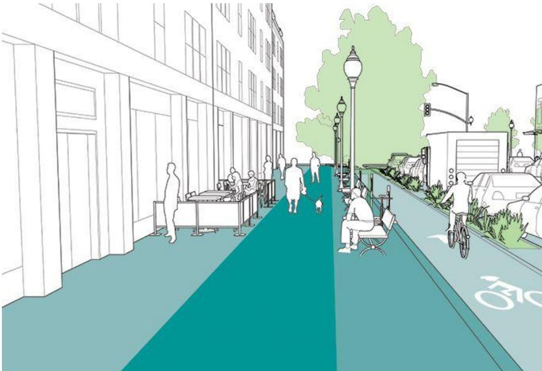
Figure 6 // The coloured areas demonstrate (from left to right) the Frontage Zone, Pedestrian Through Zone, and Furnishing Zone (NACTO Urban Street Design Guide, 2013)
